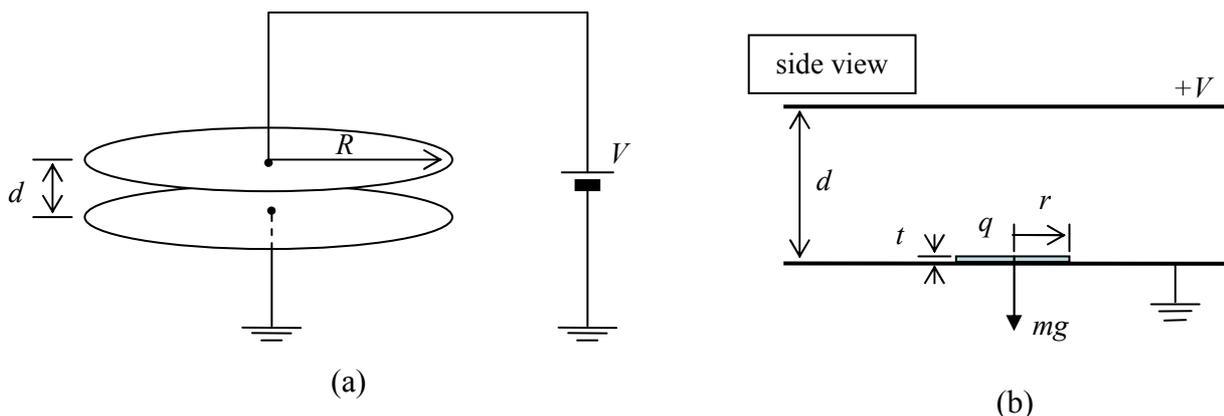
Figure 1.1 Schematic drawings of (a) a *parallel plate* capacitor connected to a constant voltage source and (b) a side view of the *parallel plates* with a small *disk* inserted inside the capacitor. (See text for details.)
